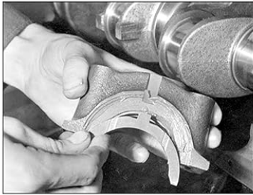
39.15 Fitting thrust washers to centre main bearing cap
