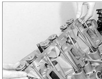
93.7a Fit the oil splash shields in position . .
