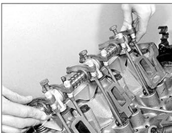
93.7b . . . and then fit the rocker shaft assemblies
