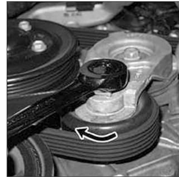
24.5 To remove the drivebelt, insert a 1/2-inch drive ratchet bar into the square hole and rotate the tensioner arm to relieve belt tension - V6 model shown, other models similar
