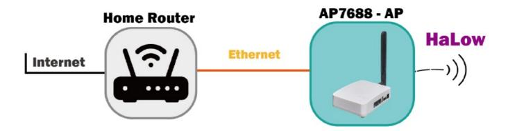
• Use CAT5 / CAT6 Cable plug in the AP mode gateway's RJ45 port.
