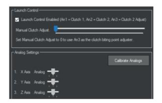
Launch Control uses Analogs 1 (clutch1), 2 (clutch2) and 3 (clutch adjustment). Manual clutch adjustment must be set to 0 to use analog 3 to adjust the biting point.
