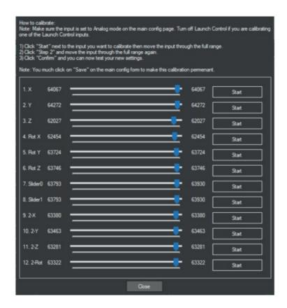
Make Sure an input is set to analog mode on the main config page. Turn off launch control if calibrating one of these inputs. Click start and move the input through the full range Click Step 2 and move the input through the full range again Click confirm and you can now test your calibrated analog. The new calibration is not saved until you click Save in the main window.
