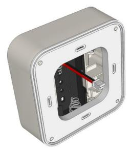
3. Insert the battery connector (See Figure 1. NUWPC3 Base Orientation and mounting, page 3, item 4) into the socket on the rear side of the module.
