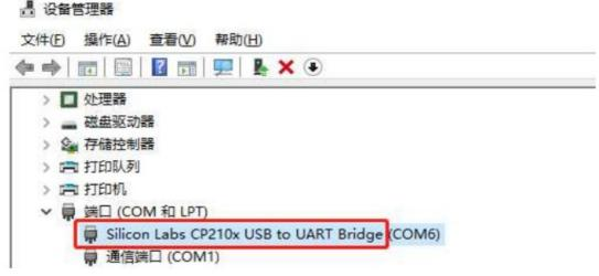
3.3If this port is not found, you need to select the corresponding driver under the "cp210x" folder for installation;
