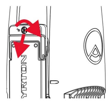
Release the Tilt lock by pulling it out and turn 90°.
