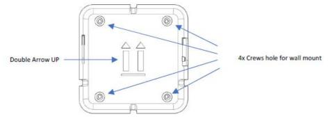
3. Attach the sensor main body to the base in the proper orientation as shown below.
