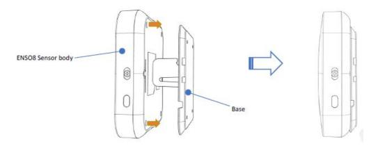
4. Slide the sensor main body down until it is locked to the base.
