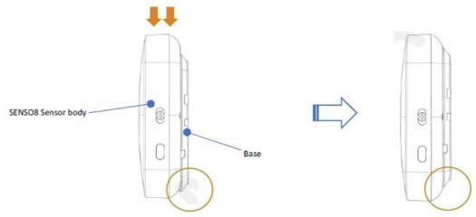
5. Lock the sensor main body with a screw.
