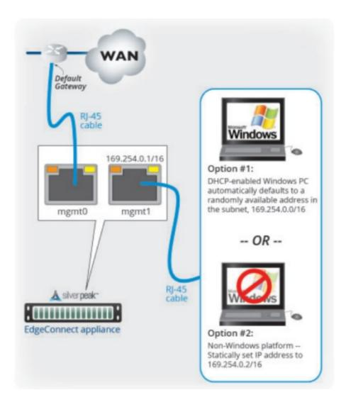
Both RJ-45 Gigabit Ethernet interfaces (MGMT0 and MGMT1) support MDI/MDI-X and auto-negotiation.
