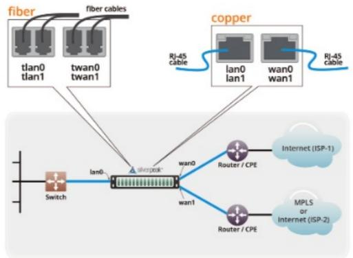
All copper RJ-45 Gigabit Ethernet interfaces in the Silver Peak appliance support MDI/MDI-X and autonegotiation.
