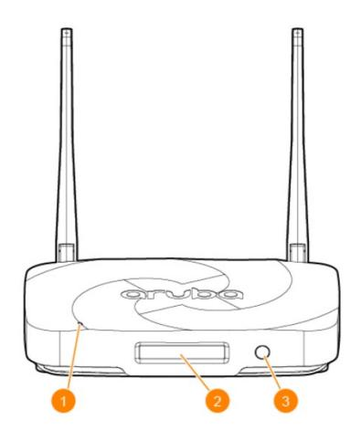
The antennas of the LTE module are in a folded position when taken out of the package. To ensure the antennas function well, put the antennas in a vertical position as shown in .
