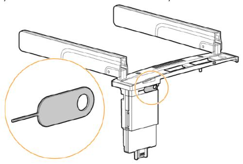
3. Insert the SIM ejector needle into the small hole on the SIM card tray. The SIM card tray will pop open.
