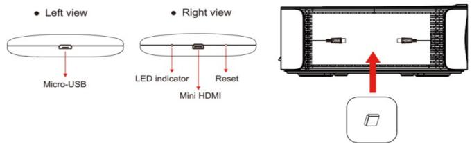
Step3. Cover the side cover to complete the installation
