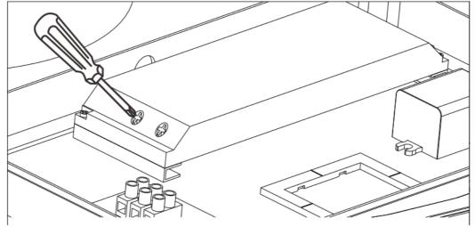
2. Remove the led driver cover, loosen screw of both led driver terminals.
