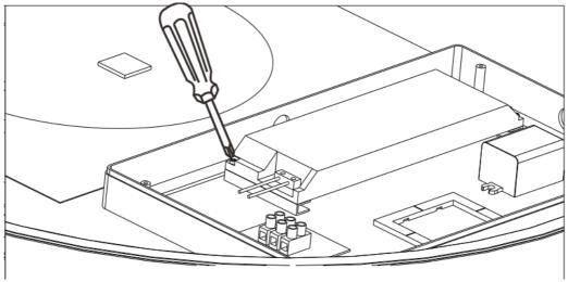
3. Remove the wires at both ends of the led driver, Unscrew the led driver base.
