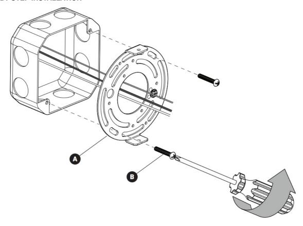
WIRES CONNECTION AND FINAL INSTALLATION
