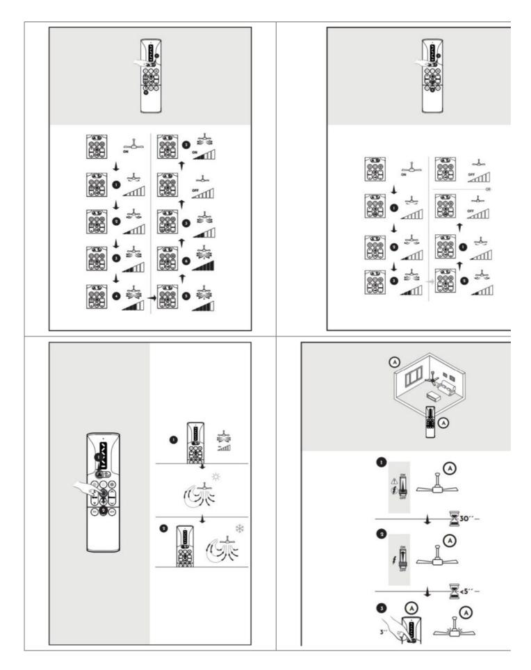
"The controller is synchronised at the factory, you only need to resynchronise the controller if you have lost synchronisation, purchased a new one or wish to control several fans with one controller.
