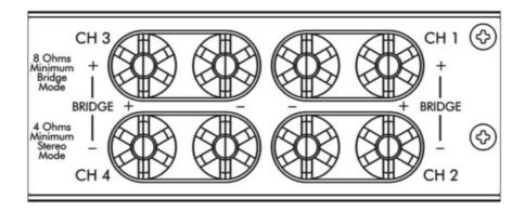
**Spade Connector** – Loosen the red and black caps on the binding posts (don't completely remove). Insert the spade connector into the binding post and tighten the caps down on the spade connector. Be sure that the connection to one post does NOT come in contact with another post.
