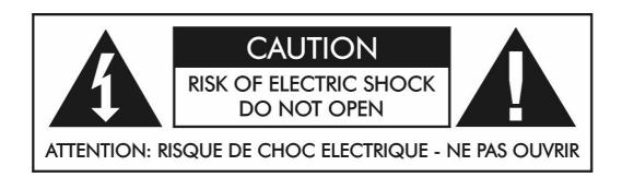
This symbol, whenever it appears alerts you to the presence of uninsulated dangerous voltage inside the enclosure voltage that may be sufficient to constitute a risk of shock.
