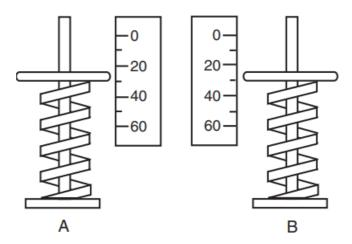
**Series PD-D Dual Switch** – Remove the front cover, held in place by two screws. There are two range-adjusting wheels. The adjusting wheel on the left (labeled A) controls the left switch, and the adjusting wheel on the right (labeled B) controls the right switch. The switches are set independently.
