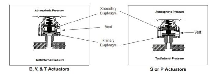
For inches of water ranges the D700, PDA, PDD and PDS switches are used as pressure switches not differential switches. The H connection is used as the process input and the L connection as the vent.
