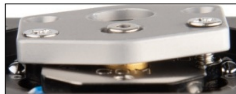
BAD: Diode improperly clamped, clip is uneven with cold plate
