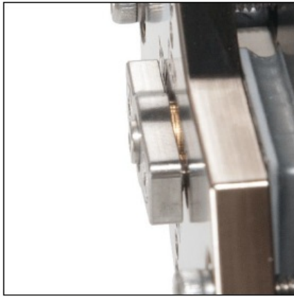
GOOD: Diode properly clamped, clip is even with cold plate
