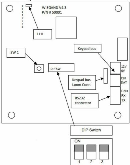
In the drawing above the DIP switches are indicating that the RS232 board is set to keypad address number 8 (switches 1, 2 & 3 all ON). Switches 4-8 are unused. To connect the RS232 V2 board to a PC or OEM device you will need to make up a serial lead. The wiring connections for that lead are shown in the table below.
