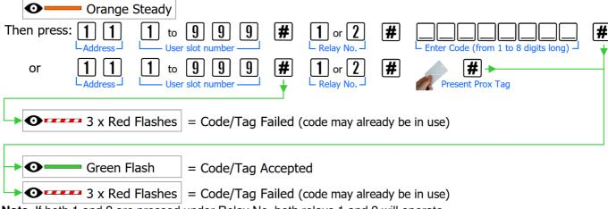
**Note.** If both 1 and 2 are pressed under Relay No. both relays 1 and 2 will operate.
