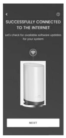
5. Your mAX router will take a tew minutes to check for new firmware, which improves system performance. If firmware is found, the LED will alternate blue and amber while downloading. If your firmware is already up-to-date or after the firmware is updated, the router will be registered. Registration ensures that you will always be running the latest and greatest firmware for maximum performance.
