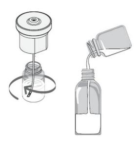
Pour a quarter inch of AromaTech Diffuser Cleaner into the empty Oil Vessel, reassemble the diffuser parts and run on the highest intensity setting for 15 minutes.
