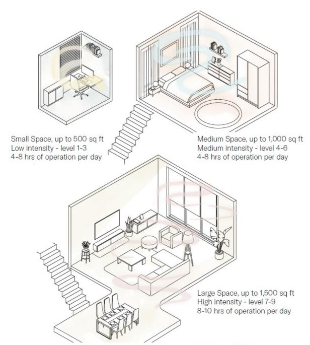
The intensity level can be adjusted from level 1 (MIN) to 9 (MAX). Start at level 1 and work your way up as needed.
