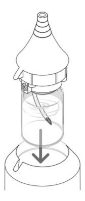
**Step 7.**Put the ceramic diffuser cover back on the diffuser base making sure the tip of the diffuser nozzle and hole in the ceramic diffuser cover match up.
