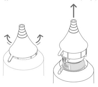
**Step 3.** Unscrew the glass oil vessel from the diffuser nozzle.
