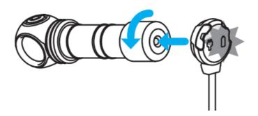
Unscrew the tailcap to 1/4 of a circle and adjust the magnetic charger to the tailcap.
