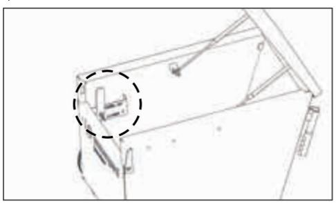
2. Moving the lever forward lowers the wheels, pulling it back will raise the wheels. Ensure the catch is properly engaged once the wheels are in position
