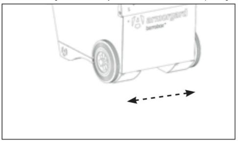
4. When the wheels are in their lower position, close the lid then use the fold-out handles on the rear of the unit to lift and push the BarroBox.
