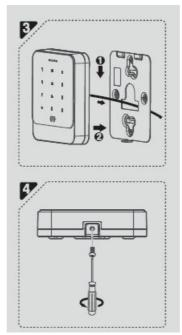
4. Fasten the device to the mounting plate with a security screw
