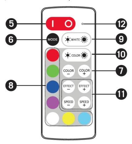
Mode selection Press this key to switch between RGB, white, and RGB+white mode. If the RGB mode is selected, the white channel will be disabled, and if the white mode is selected, RGB channel will be disabled. In RGB+White mode all channels are enabled.
