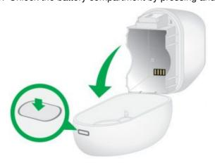
2. Gently pull the battery door back to open the compartment.
