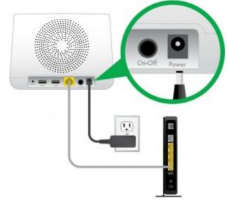
3. Turn the base station on by pressing the **On/Off** button.
