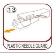
(13) PLASTIC NEEDLE GUARD. Remove the stylus by pulling it straight down and out, in the opposite direction of the tone arm.
