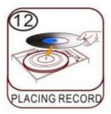
(12) PLACING RECORD Put records corresponding to the turntable, Lift the pickup and place it lightly on the record, You can play the songs from the record
