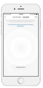
3. Put the device close to your phone. Press and hold the button until the device beeps. The app will detect the device automatically.
