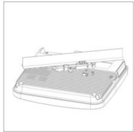
3. Place the first mounting post on the rear-side of the AP on to the lower notch of the bracket.
