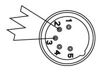
A DMX512 terminator reduces signal errors, avoiding most signal reflection interference. Connect PIN 2 (DMX-) and PIN 3 (DMX+) of the last fixture in series with a 120 Ohm, 1/4 W Resistor to terminate the DMX512.
