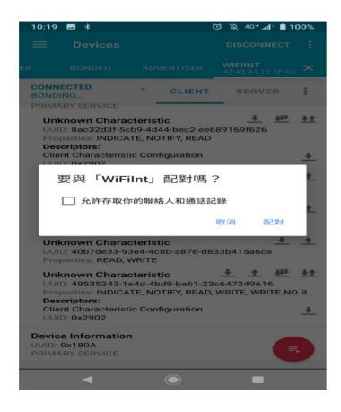
5. Click Unknown Characteristic in the Unknown service, UUID was 40b7de33-93e4-4c8b-a876-d833b415a6ce, click button "Write" to process and setting wifi password, see below illustration
