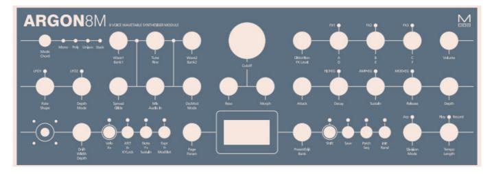
Preset/Edit/Bank – This encoder/switch is used to adjust the value or 'trigger' the currently displayed parameter. When on the 'Load Patch' parameter when the panel is in 'Shift' mode this encoder is used to select the patch bank number.
