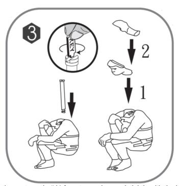
After assembled #40, insert the center pole #41 from top and screw it tightly with the key included.
