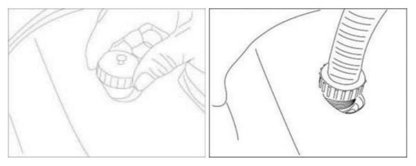
• Open the air valve on the whirlpool cover and attach the filling hose to the valve.
