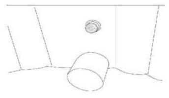
Remove the filter cartridge cover.
