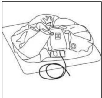
• b. Open the air outlet on top of the filter heating element of the whirlpool and screw on the filling hose.
