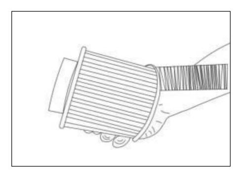
Place the filter cartridge cover on the new filter cartridge and screw it in by turning it clockwise.
