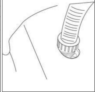
• c. Open the air valve on the whirlpool cover and attach the filling hose to the valve.
