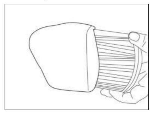
The filter cartridge can be rinsed off with a garden hose and reused. However, if the filter cartridge is dirty and discolored, the filter cartridge should be replaced.
