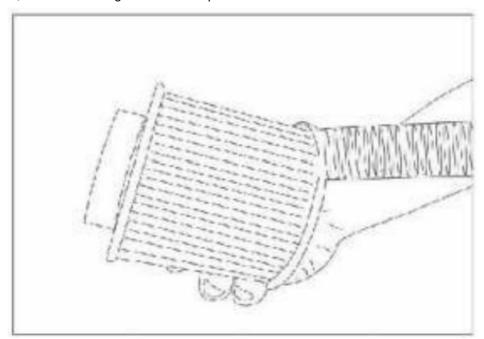
• Place the filter cartridge cover on the new filter cartridge and screw it in by turning it clockwise.
