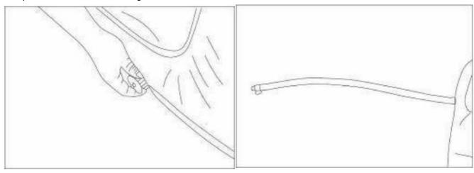
Then pull off the plastic plug on the inside. Now the water can flow out. When the spa is out of water, press the BUBBLE button for 2-3 minutes to drain the water in the air line. When the water is completely drained, remove the filling hose and close both outlets again.
