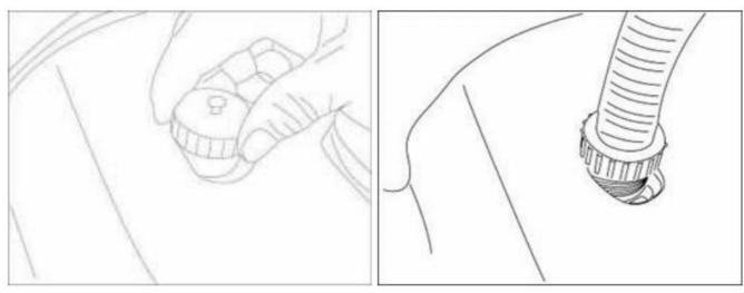
• Open the air valve on the whirlpool cover and attach the filling hose to the valve.
