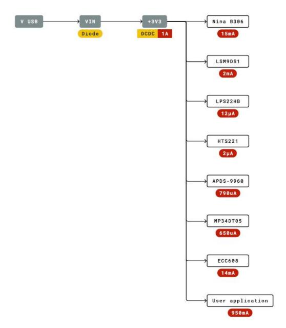
**NOTE:** Since VUSB feeds VIN via a Schottky diode and a DC-DC regulator specified minimum input voltage is 4.5V the minimum supply voltage from USB has to be increased to a voltage in the range between 4.8V to 4.96V depending on the current being drawn.
