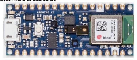
Nano 33 BLE Sense is a miniature-sized module containing a NINA B306 module, based on Nordic nRF52480 and containing a Cortex M4F, a crypto chip which can securely store certificates and pre shared keys and a 9 axis IMU. The module can either be mounted as a DIP component (when mounting pin headers), or as a SMT component, directly soldering it via the castellated pads
