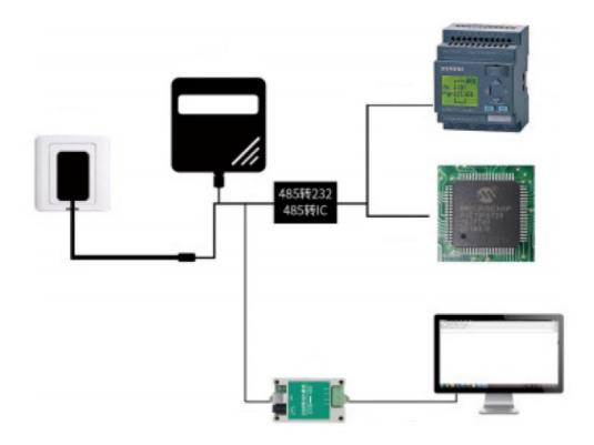
This product can also be used in combination of multiple sensors in a 485 bus. In theory, a bus can have 254 485 sensors, the other end is connected to a PLC with a 485 interface, a single-chip microcomputer is connected through a 485 interface chip, or a USB to 485 can be used to communicate with the Computer connection, use the sensor configuration tool provided by our company for configuration and testing (only one device can be connected when using this configuration software).
