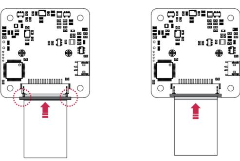
4. Connect the camera to Raspberry Pi, with pins facing away from the catch.
