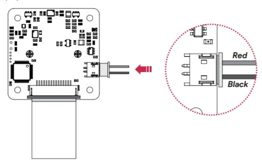
6. Connect the 2-pin cable to Raspberry Pi's GPIO (5V & GND).
