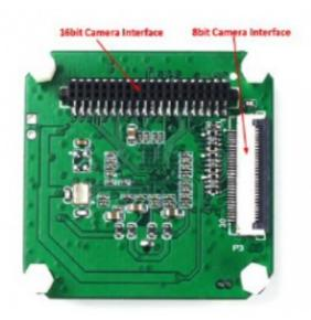
There are two camera interface provided on the USB3 camera shield, but only one camera interface can be used at a time.
