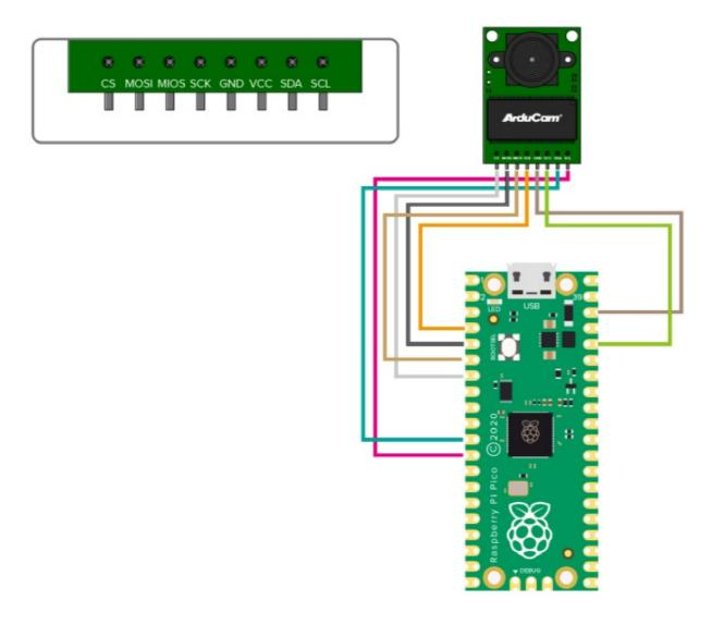
**NOTE**: Arducam Mini 2MP camera module is a general-purpose solution compatible with multiple platforms, include Arduino, ESP32, Micro:bit and the Raspberry Pi Pico we're using. For the wring and software on other platforms, please refer to the product page: <a href="https://www.arducam.com/product/arducam-2mp-spi-camera-b0067-arduino/">https://www.arducam.com/product/arducam-2mp-spi-camera-b0067-arduino/</a>
