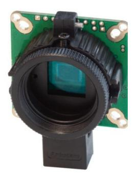
This Arducam IMX477 High-Quality Camera board is designed for Raspberry Pi, no lens is included in this product, and we recommend you use a C- or CS-mount lens with it.
