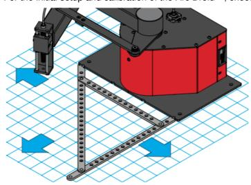
2. Place the Arc Droid™ on the work surface with a clear area in front and to the sides of the machine to allow for arm movement.
