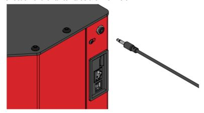
Plug the calibration sled into the connection on the side of the ArcDroid™.
