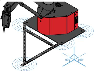
Attach the stylus to the Z-axis plate and secure with the locks. Do not plug into the Arc Droid™.
