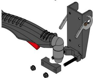
Insert the torch into the torch mout, and align the body of the torch handle to be approximately parallel with the torch mount.
