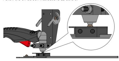
The universal torch mount can be removed and reinstalled from the ArcDroid™ without the need to recalibrate, as long as the cutting head remains firmly attached to the universal torch mount.
