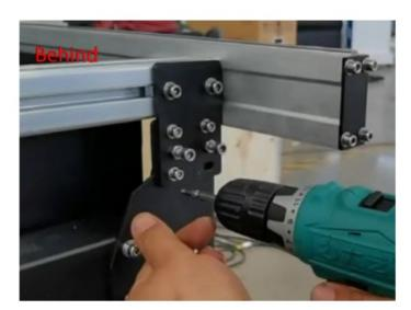
The Y axis Frames and tracks assembled:
