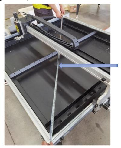
The diagonal of the device is adjusted to ensure the perpendicularity of the X and Y axes;
