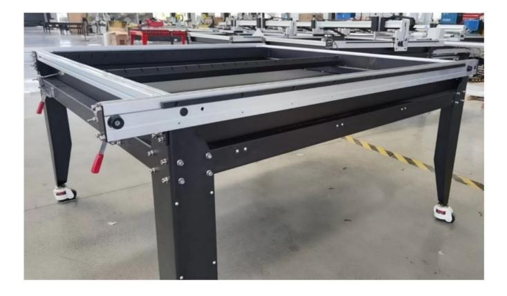
Step 4: Install X axis Frames and tracks to Y axis Frames.
