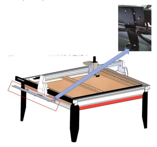
2. Remove the drag chain from the beam; The the drag chain are fixed in the X-axis drag chain groove and the Y-axis the drag chain groove respectively
