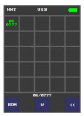
• To do this, select a single cell (highlighted with a white border) and press the "ROM" button, you will be asked to write the information to the internal memory of the device. The stored cell will be displayed with the "\*" icon. Pressing the "W" button returns the information back to the home screen.
