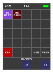
• The device provides a mode for automatically transferring all currently detected signals to the "white" list. To do this, on the main screen, without selecting a specific cell, press the "W" button. You will be asked to start the automatic detection mode and transfer signals to the "white" list.
